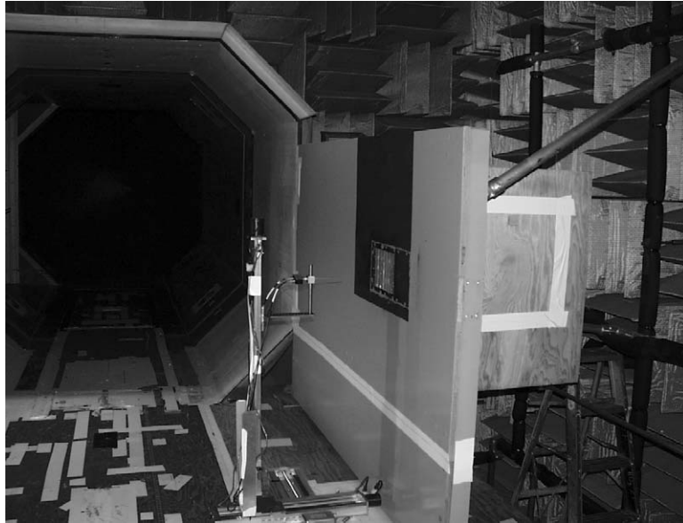
Fig. 4. Photograph of test plate and cavity installed in the wind tunnel. View is looking upstream from anechoic section into closed jet section. Traverse system and probe support are visible in front of the cavity opening.
